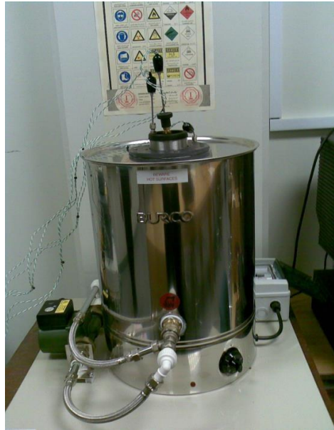
Figure 1: Unsteady heat transfer experimental unit
