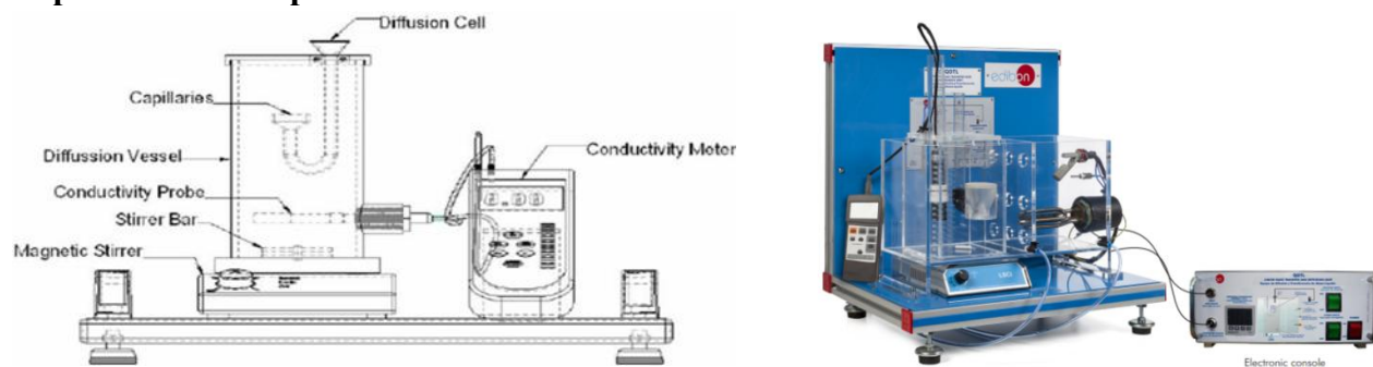
Fig 1. (a) Schematic diagram of mass diffusion experimental setup and (b) Picture of the setup.
